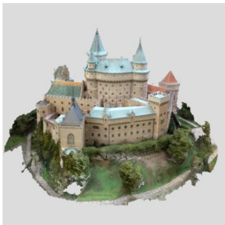
Fig 26 e 27 - Photogrammetry 3D from a Castle, resource from camera capture with stereo 3D Capture device
