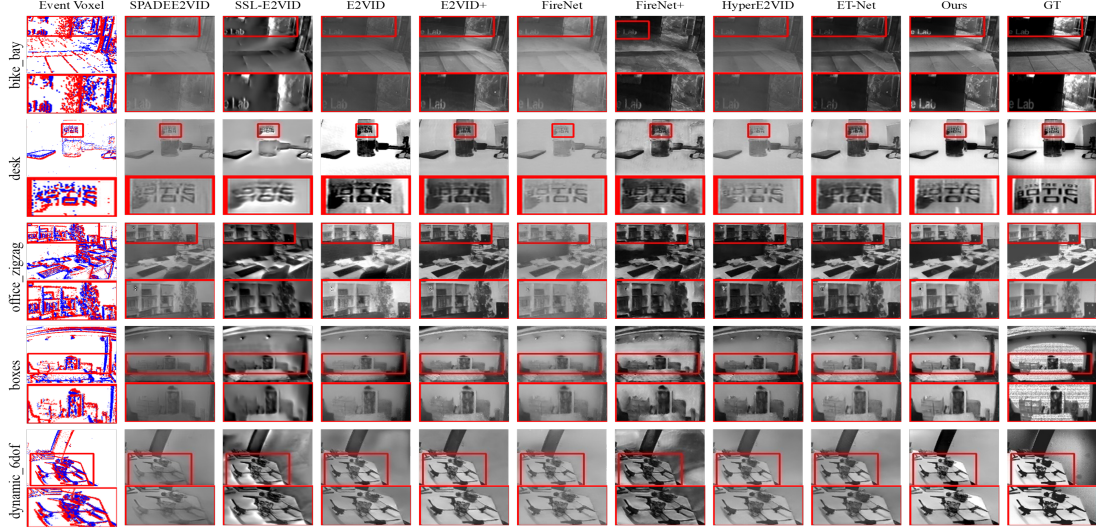
Fig. 3. Visual results on HQF (rows 1 and 2), ECD (rows 3 and 4), and ECD_fast (last row). We provided a magnified view of each reconstructed scene where visual differences are more prominent. Overall, our reconstructed scenes are more close to GT images in terms of contrast and fine details.
