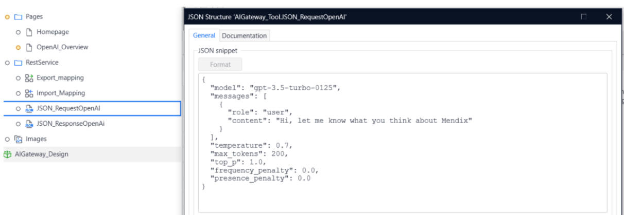
Figure 28 - Request body of the Post Completion method in the exposed REST API using Mendix
