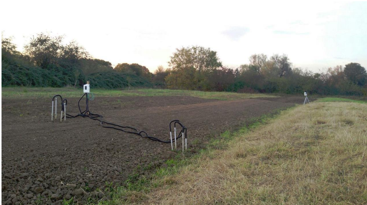
Weather station with soil sensors (measuring soil humidity and moisture from 0-90cm in the ground) on the experimental ridge and furrow fields of the Open-Air Laboratory Lauresham. Source: Staatliche Schlösser und Gärten Hessen.
