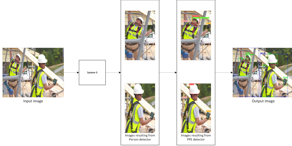
Fig. 4 Overview of System 3: A two-stage detection process with image cropping for enhanced precision.
