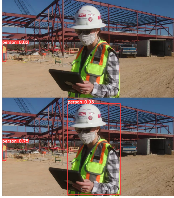
Fig. 5 Comparison of person detection performance. The upper part of the image shows the detection result of the trained YOLOv8 model, which fails to identify the person. The lower part of the image shows the detection result of the default YOLOv8 version, which successfully detects the person (highlighted in a red bounding box).
