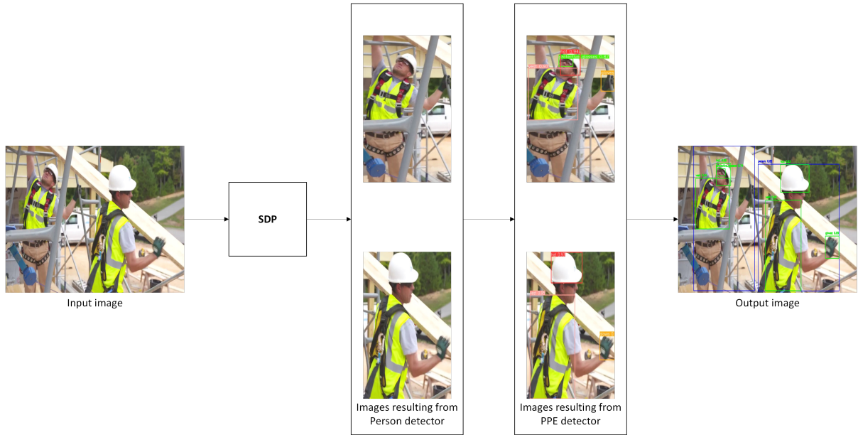
FIGURE 7. Overview of SDP: A two-stage detection process with image cropping for enhanced precision
