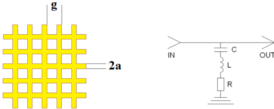
Figure 9 – Inductive metallic mesh structure and its equivalent circuit model, adapted from [8].
