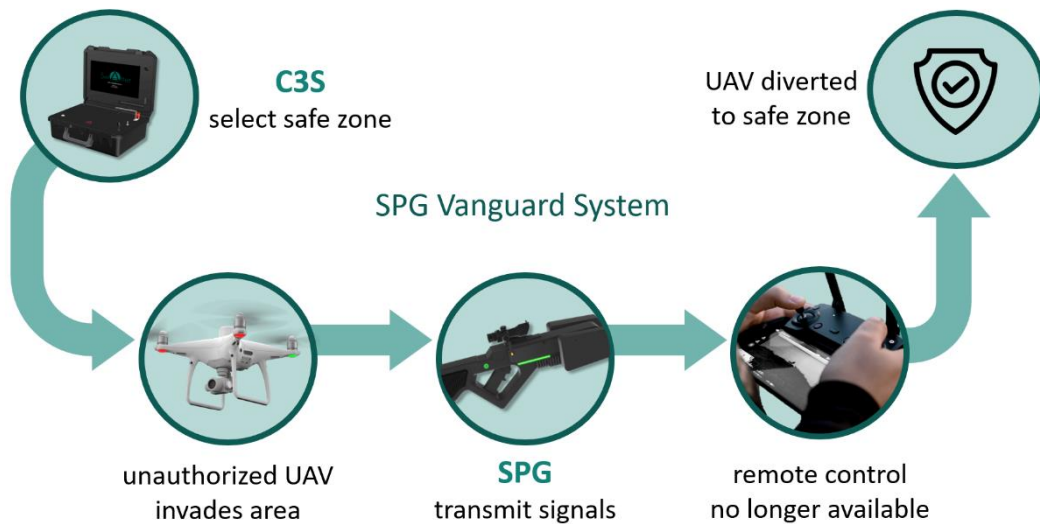
Figure 4.11. How SPG Vanguard System work
