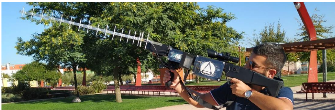
Figure 5.7. Unauthorized drone protection system
