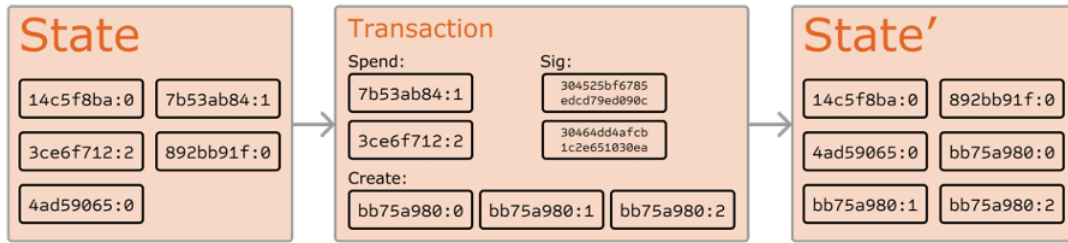
FIGURE 1. Illustration of state changes with new transactions on the Bitcoin Network
