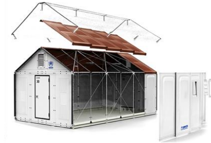
Figure 14 | How an RHU is assembled
