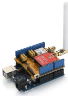
FIGURE 3.6: Arduino and Lora Shield connected
