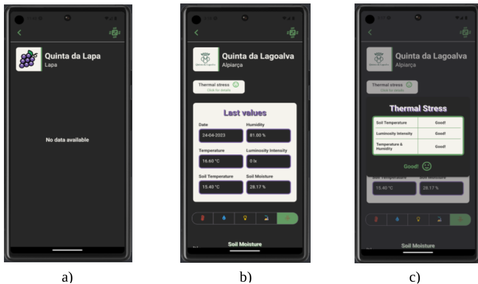
Figure 4.10 - Mobile Application Vineyard Dashboard; a) No Data Available; b) Last Measured Values; c) Pop-up with Thermal Stress Status
