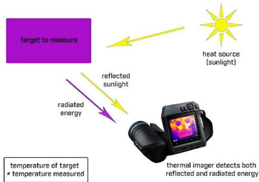
Figure 2.7 - Effects of solar emissivity in thermal imaging
