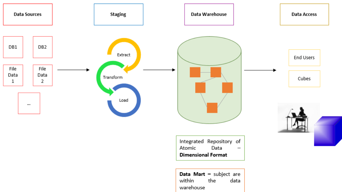
Figure 22 - Data Warehouse Architecture (Kimball) – adapted from Adamson (2010)
