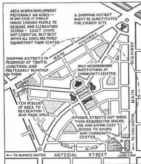
Fig. 3 – “Neighbourhood Unit” diagram, according to Clarence Perry, 1928. (Source: New York Regional Survey, vol.7, 1929)
