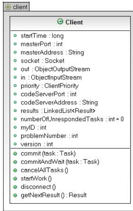
Figure 19: Class diagram - Client class
