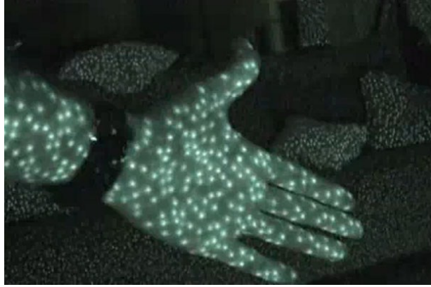
Figure 4 - The projection of a computer-generated hologram on the environment by Kinect.
