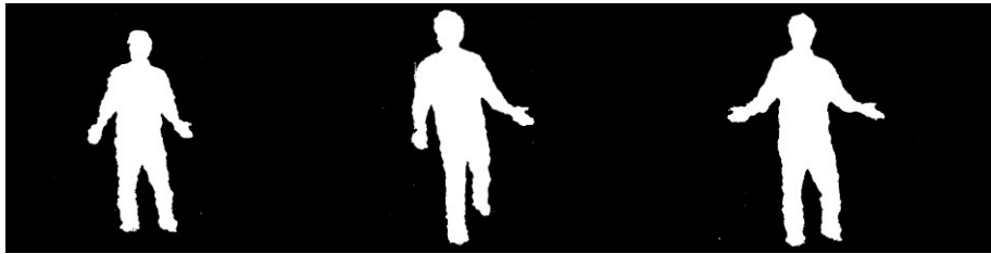
Figure 8 – With background subtraction, the body silhouette becomes the only visible object as it moves around the sensor field of view.
