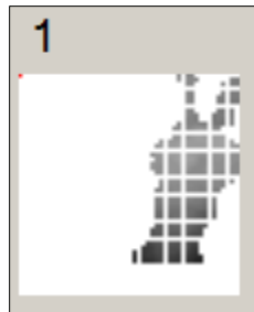
Figure 12 - Lack of dexel information when scaling or when the hand is far away from sensor field of view.
