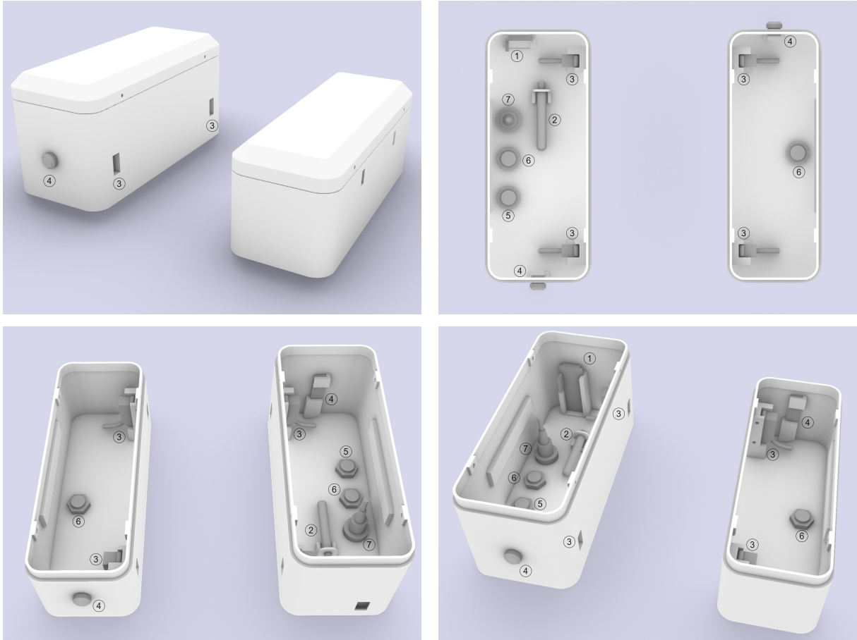
FIGURE 3.9. Overview of the developed sensor enclosure prototype: (1) microcontroller, (2) microcontroller LoRaWAN antenna, (3) AIR, (4) PIR, (5) panel connector 2 PIN, (6) panel connector 5 PIN, (7) panel micro USB adapter
