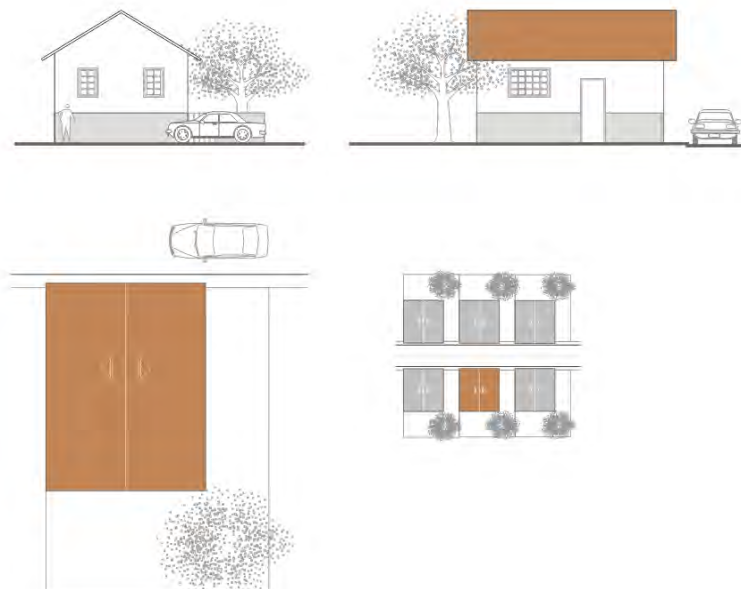
Figure 31. Isolated type . Schema of façades, building implantation and situation. Characteristics: frontal façade on the alignment of the street; entrance door on the lateral façade; lateral and back spacings; roof of ceramic tiles, with two inclinations and small edges. (Source: schemas produced by the authors, no scale).
