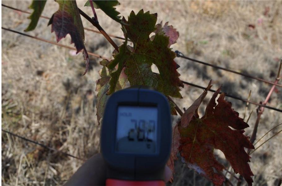
FIGURE B.5. Measurements of Leaf Temperature to Establish CWSI Parameters
