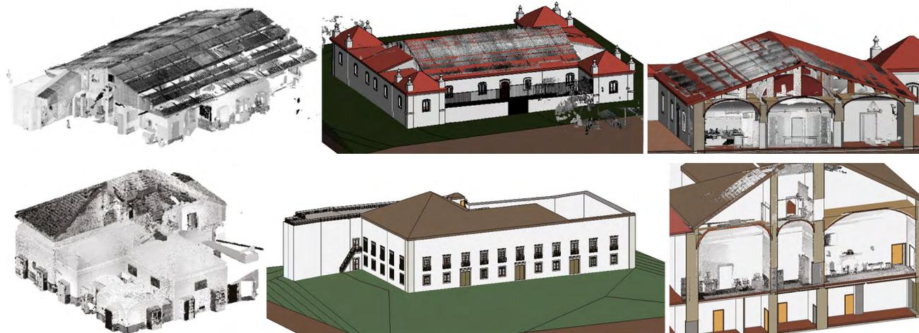
Fig. 4 3D models of the Quinta de São Brás house in Serpa: Point clouds with TLS (left) and compatibilisation of point clouds with BIM model (centre and right). Source: Folgado 2024,34, 44.
