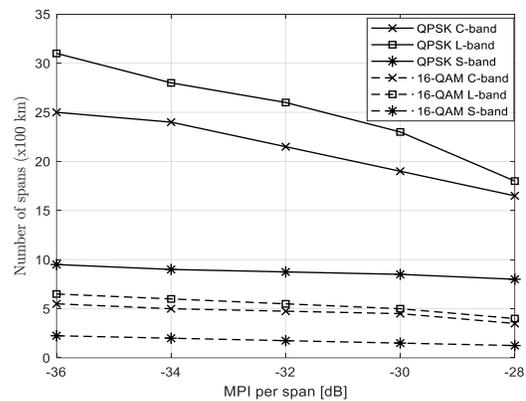
Fig. 2. Number of spans as a function of the MPI level per span for the three bands and for QPSK and 16-QAM signals.
