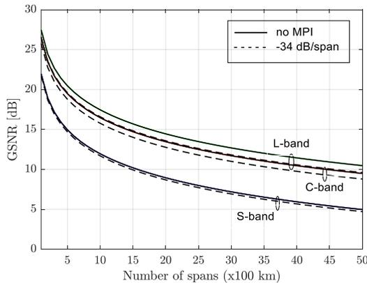
Fig. 1. GSNR as a function of the number of spans for the three bands and two MPI scenarios – no MPI and -34 dB/span.
