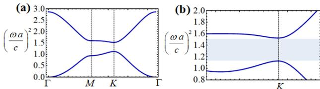
Figure 2: (a) Photonic band structure of the ferrite photonic crystal. (b) Zoom in of panel (a) around the  $K$  point.
