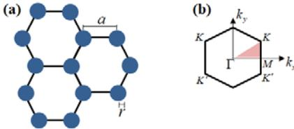
Figure 1: (a) Hexagonal array of ferrite cylinders. The distance between nearest neighbors is  $a$ . (b) First Brillouin zone of the 2D lattice.
