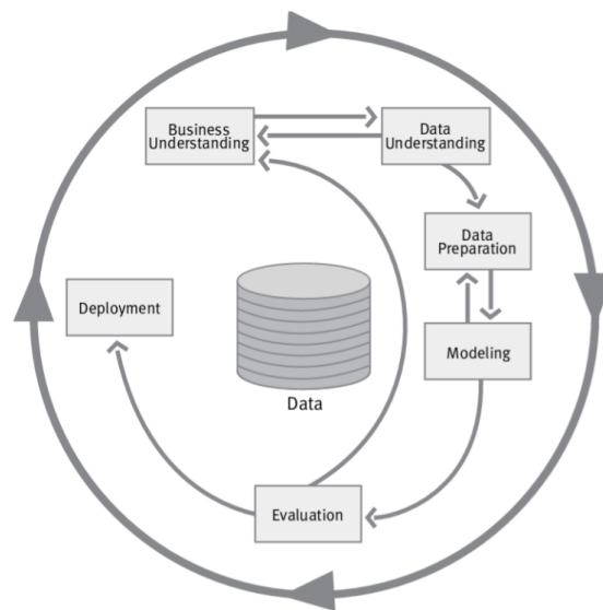
FIGURE 1.1. Phases of the CRISP-DM reference model. Figure reprinted from [6].
