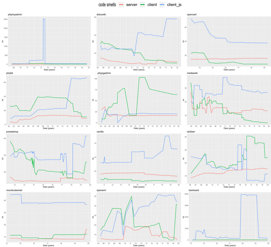
Fig. 5 Evolution of Code Smell groups in web apps (Y axis: CS density by LOC ; X axis: years)
