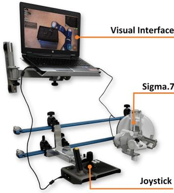
Fig. 3: Setup for ANALOG-1 teleoperation experiment [4].
