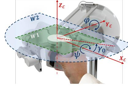
Fig. 6: Sigma workspace ( $W1$ : actuation area,  $W2$ : saturation area), Cartesian frame ( $X_C, Y_C, Z_C$ ), wrist offset ( $\gamma_0$ ), and haptic feedback ( $\psi$ : roll,  $\varphi(t)$ : pitch).
