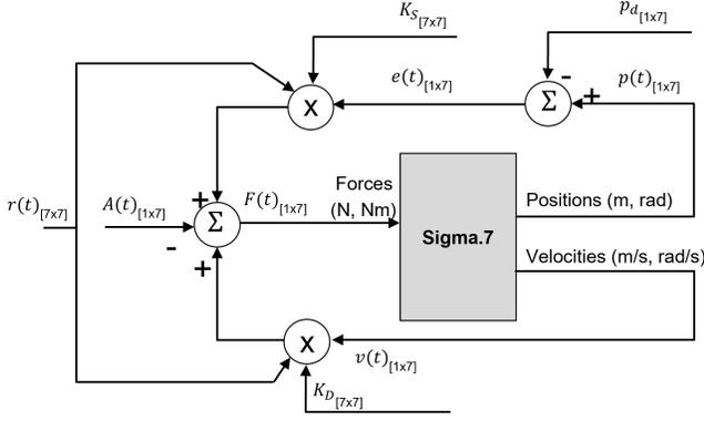
Fig. 5: Control loop implemented to control sigma.7 (see Section II-A for the notation used).
