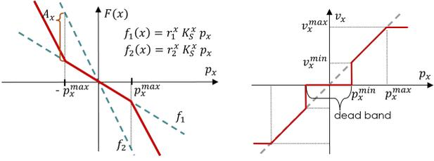
Fig. 7: Implemented force Fig. 8: Actuation rendering profile (full red line, Eq. 4). (mapping  $p_x$  and  $v_x$ , Eq. 9).
