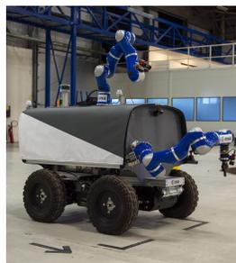
Fig. 1: Interact rover: four-wheel-steering mobile platform [4].
