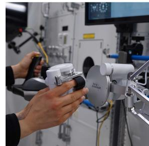
Fig. 2: Operator holding sigma.7 device while it displays the rover’s pitch.
