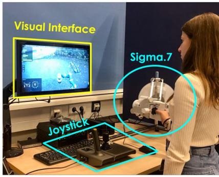
Fig. 9: Apparatus: Teleoperation Station with the visual interface, sigma.7 and joystick.
