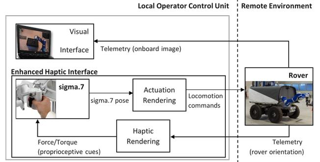
Fig. 4: System architecture and its main components: “haptic rendering”, “sigma.7”, and “actuation rendering”.
