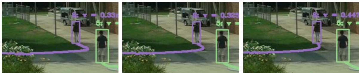
Figure 4.12. Examples of applying the trajectory smoothing process on a sharp turn: 5-point window (left), 8-point window (middle), and 10-point window (right).
