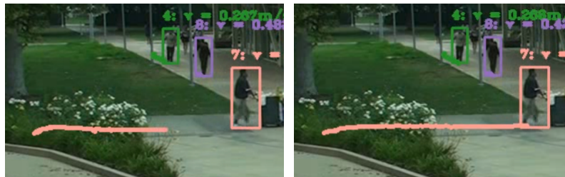
Figure 4.11. Examples of applying the smoothing process (10-point window) using: only past trajectory information (left), and both past and future trajectory information (right).
