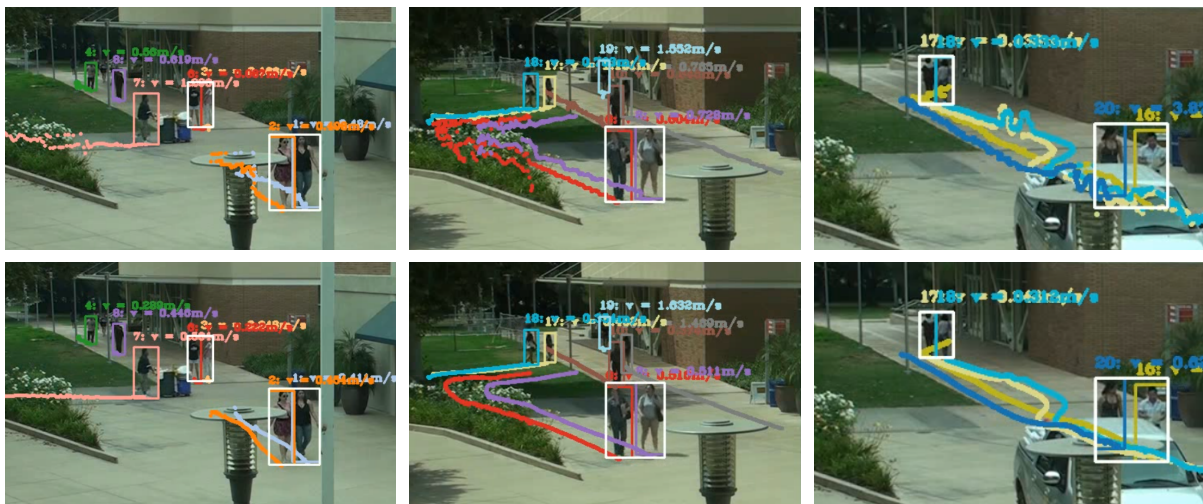
Figure 4.14. Examples of applying the proposed trajectory smoothing method (with occlusion awareness): without trajectory smoothing (top) and with trajectory smoothing (bottom).
