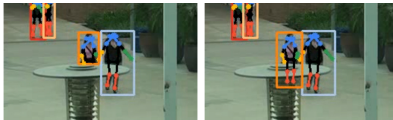
Figure 4.10. Example of reapplying the HRNet algorithm to the corrected bounding boxes (only joints with a confidence score over the threshold of 0.3 are drawn): before occlusion awareness (left) and after occlusion awareness (right).
