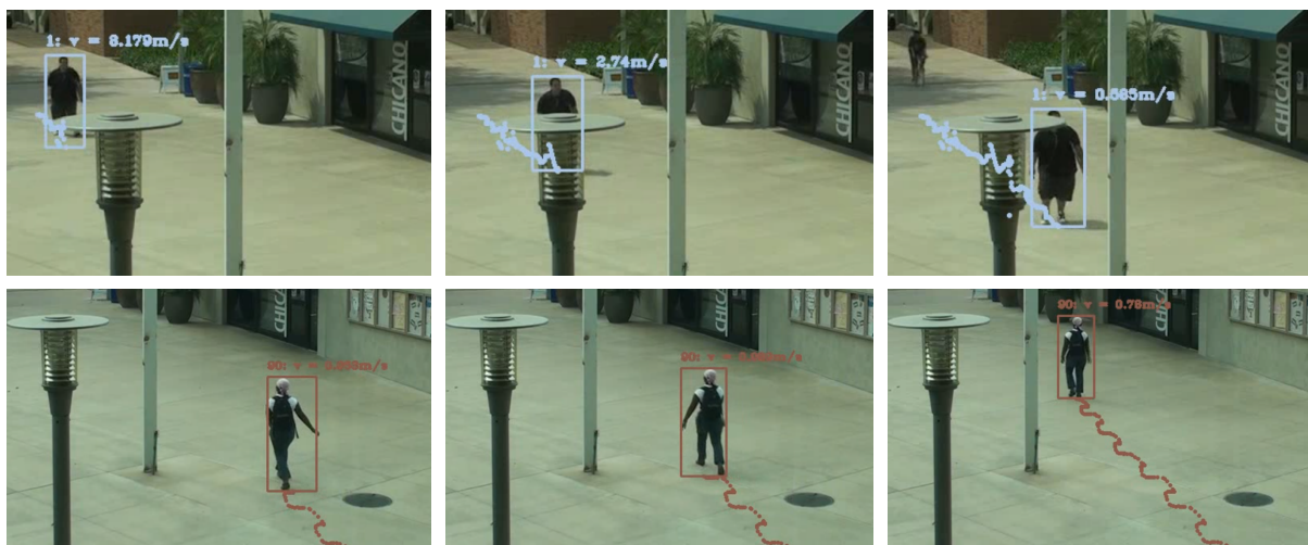
Figure 4.6. Examples of the two major factors that create irregularities in the extracted trajectory points: occlusions (top) and gait movement (bottom).
