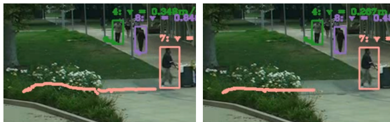
Figure 4.7. Example of applying the trajectory smoothing method to irregularities caused by obstacles: 5-point window (left) and 10-point window (right).
