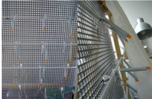
Figure 5. Morphosis prototype without membrane and its SMA levers
