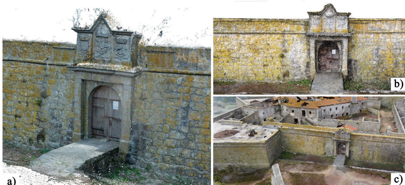
Figure 9. a) Perspective view of the point cloud of the fortress entrance, obtained from the SfM processing of 256 photos taken with a digital camera. On the right 3D, model obtained from 108 aerial photos (b – dense cloud, c – model 3D textured).
