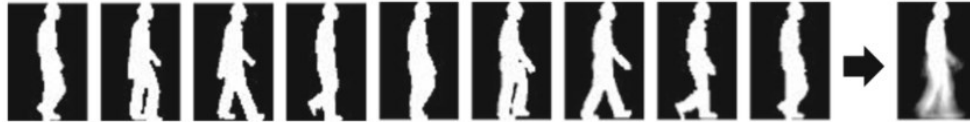
Figure 6 - Gait sequence through a series of key silhouettes, and the resulting Gait Energy Image (GEI), taken from [32]
