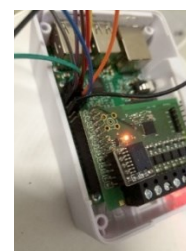
Fig. 3. Raspberry Pi with SensFloor shield
