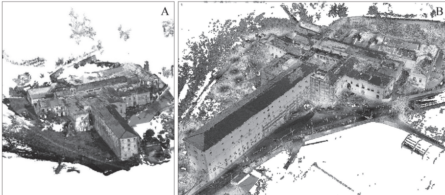
Fig 5. (A) Dense Point Cloud from Photogrammetry; (B) Junction of the 3D Point Cloud of Photogrammetry and Laser Scanning.
