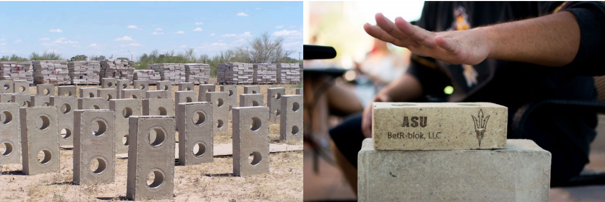
Image 1.11 – a) Various paper bricks to be used for construction are displayed and b) a smaller prototype example of the paper brick from the BetR-Block company (Jones, 2016).
