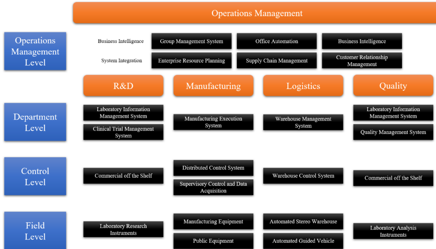
Figure 2 Intelligent Manufacturing System Framework for Pharmaceutical Companies (Developed by MIIT & CEPA (2020))
