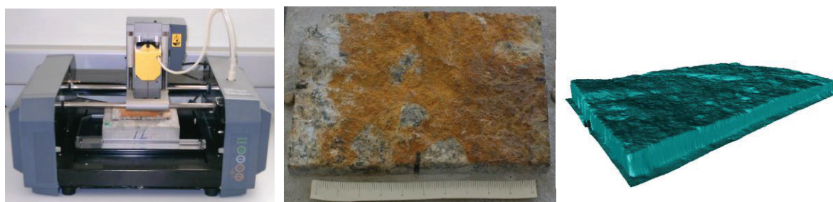
Fig. 1. The scanner with a joint specimen positioned with the Perspex frame, the surface of a rock joint and its corresponding digital image rendered by the scanner control software.
