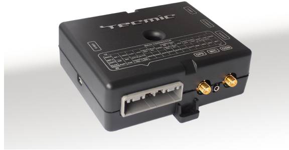
Fig. 4. XTraN's on-board processing unit for monitoring vehicle [22]
