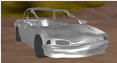
Figure 2. Deformed car after a violent impact
