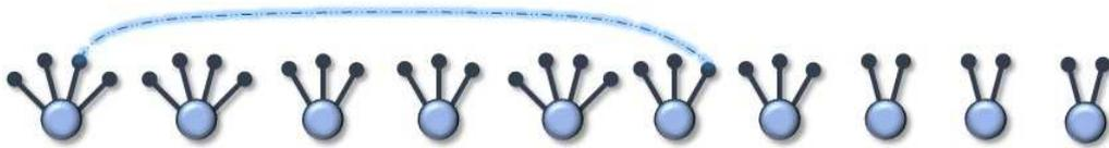
**Figure 3.2. Wiring the configuration model.** Example of setting up a first link between node stubs for a network with  $n = 10$  nodes, 15 links and degree sequence  $D = \{4, 4, 3, 3, 4, 3, 3, 2, 2, 2\}$ . Stubs are randomly chosen and as long as  $\sum_{i=1}^n D_i$  is even, the process always concludes, albeit with multi links and self loops.
