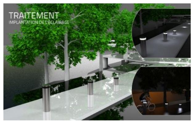
**Figure 11.** Graphic representations of the development proposal of group n°1 (Baugé and Charrière). The synthetic images show luminous devices of the bollard type, whose height decreases as the path progresses in the forest. These simulations show a daytime view (left) and two nighttime views (right). © Baugé and Charrière
