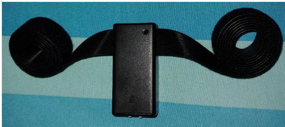
Figure 20 – Final Prototype of the Respiratory Rate Sensor. This prototype consists of a module that includes the use of sensors and mechanisms in order to estimate the respiratory rate in real-time. Furthermore, a Velcro strap was chosen instead of the typical elastic bands, which gives more rigidity, but more flexibility in the adjustment.
