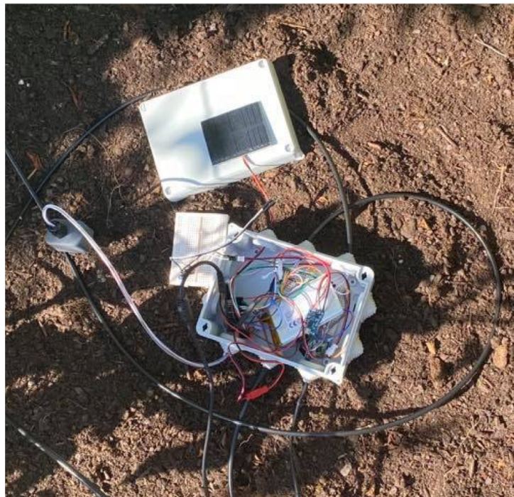
FIGURE 6.9. Irrigation Management Traditional Sensor Node [128]
