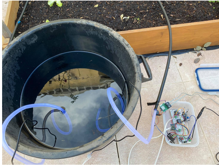
FIGURE 6.13. System Implementation—Actuator Node [128]
