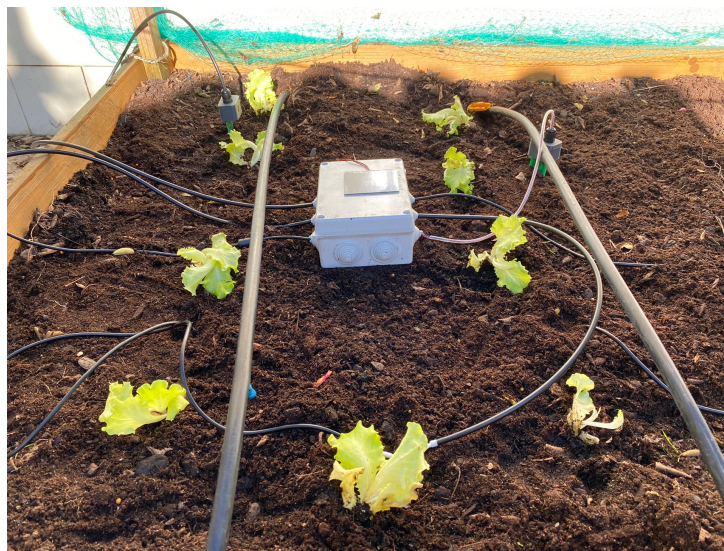
FIGURE 6.12. System Implementation—Sensor Nodes [128]
