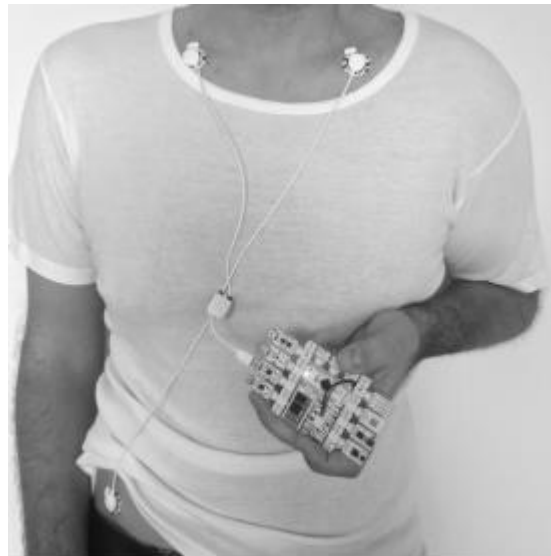
Fig 4.1 - ECG electrodes position [35]
