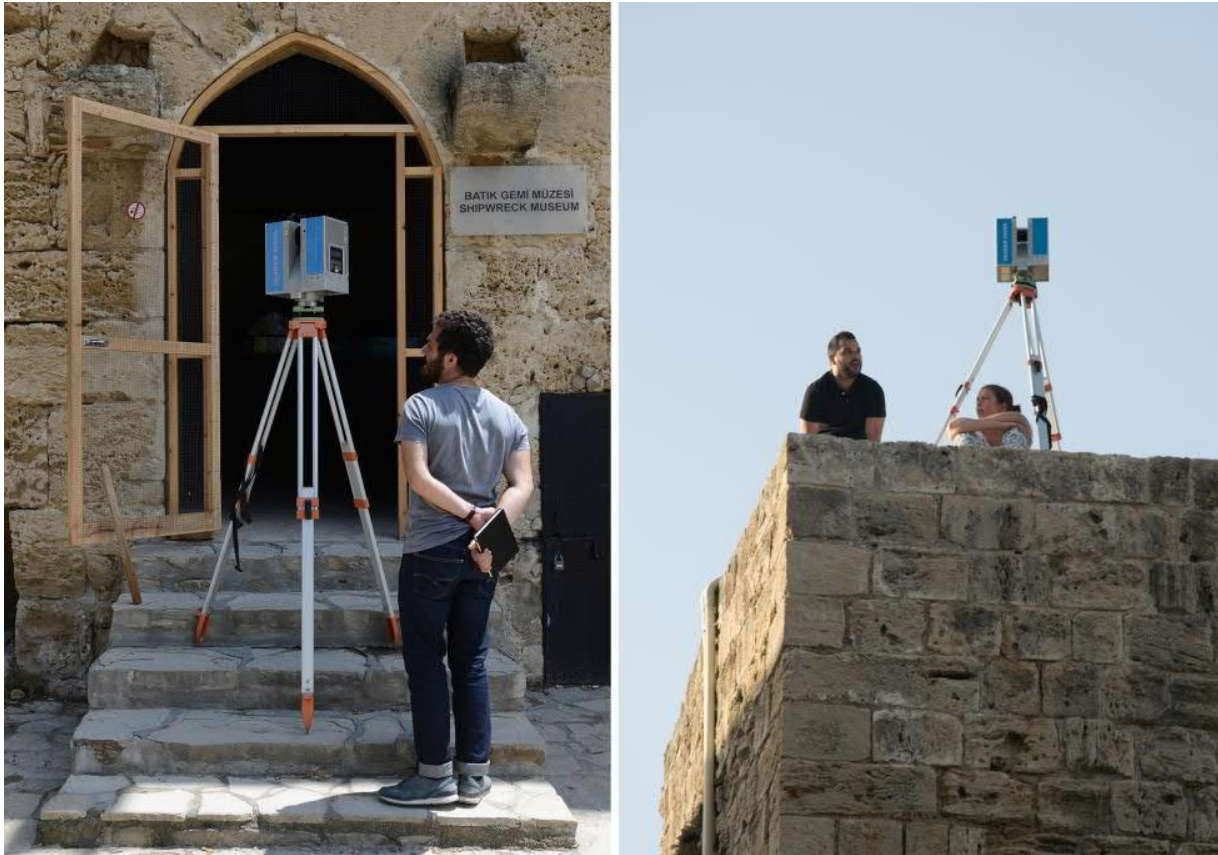
Fig. 5. Representative picture of the digital survey campaign carried out with a laser scanner Z+F IMAGER 5006h
