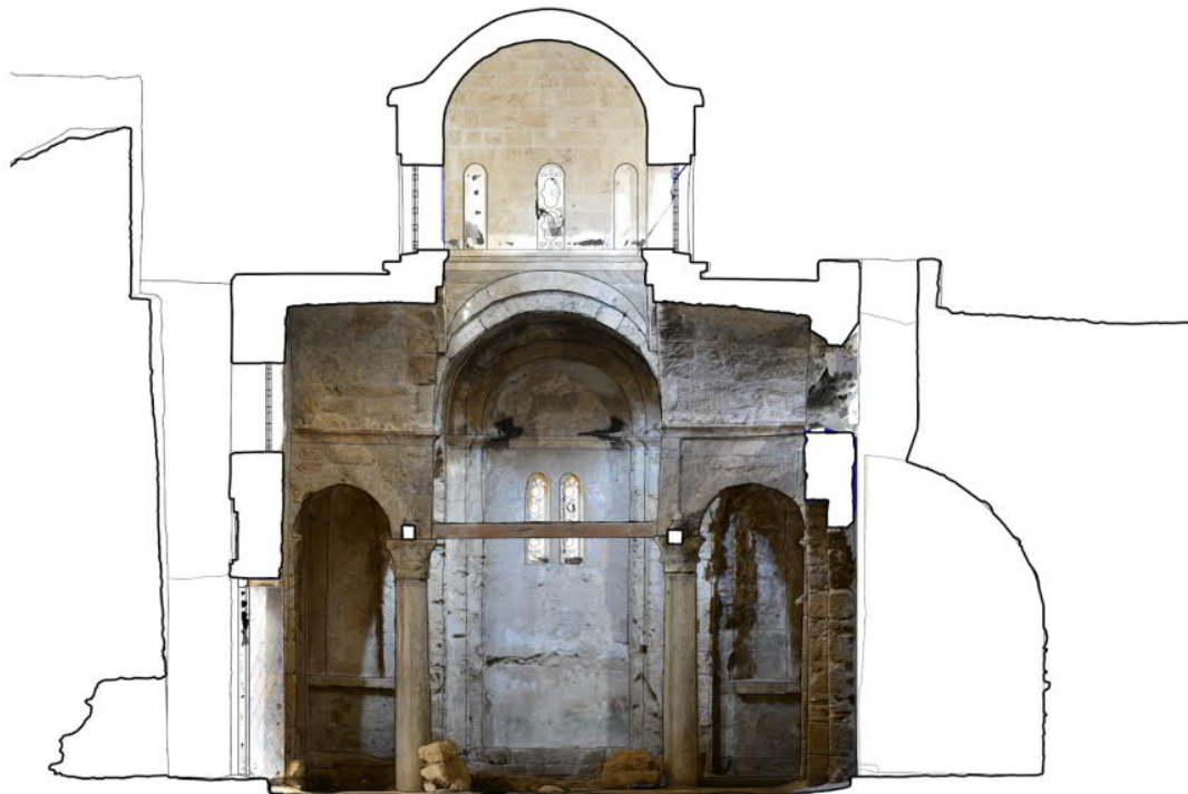
Fig. 13. Final drawing of a 2D section of the church with the ortophoto taken from the 3D model
