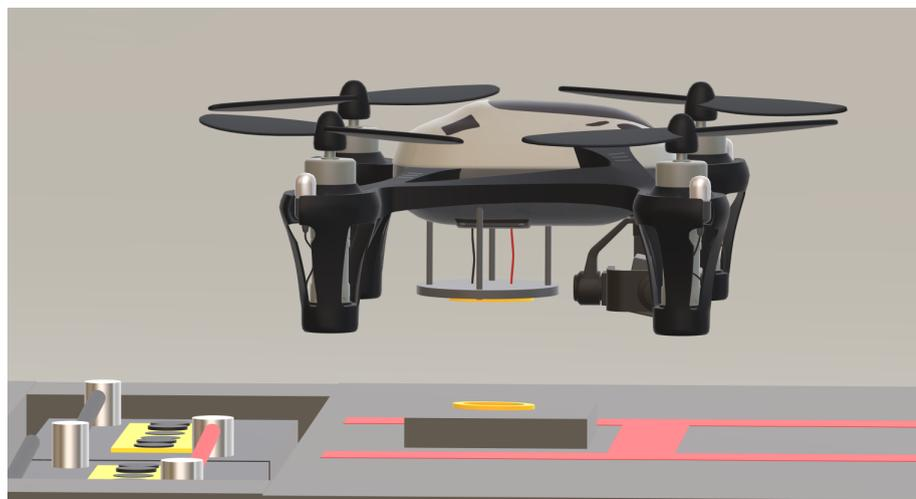
FIGURE 5.16: UAV and base WPT recharging system.
