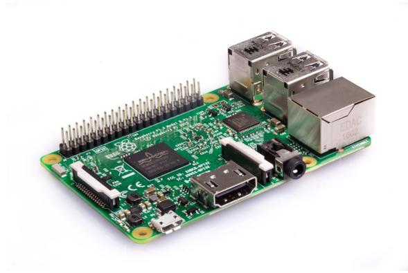
FIGURE 2.8: Raspberry Pi board.
