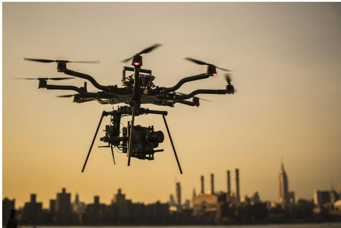
FIGURE 2.5: Multi-Rotor MAV.
