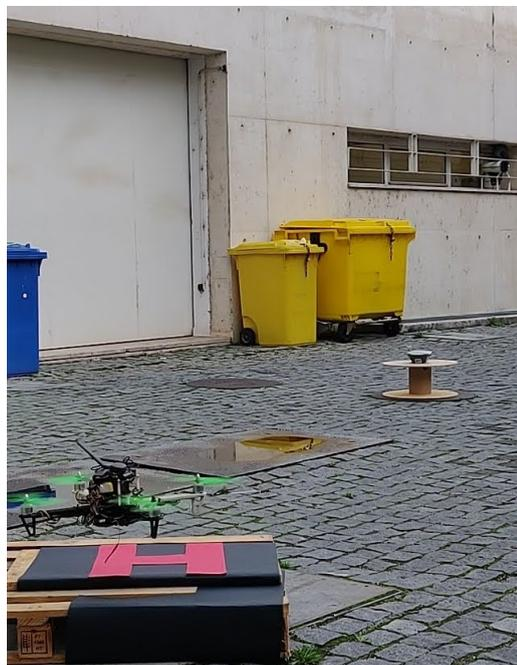
FIGURE 6.14: High precision landing testing.
