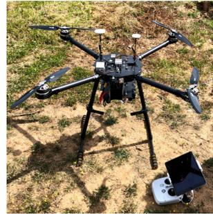
Fig. 3. Quadcopter UAV, the RC controller and the visual interface (tablet).
