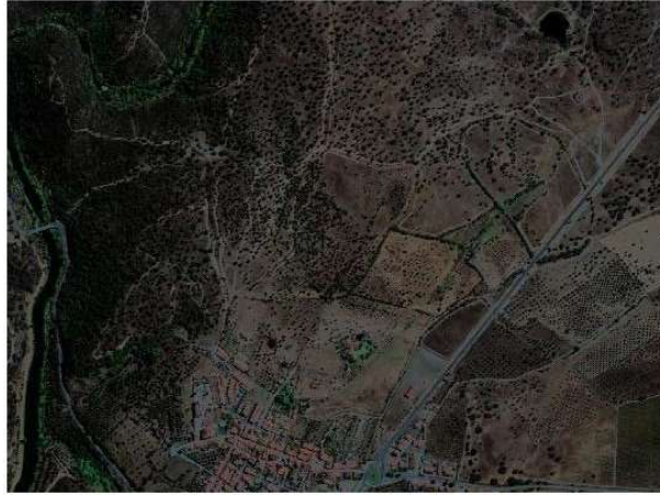
Figure 27: Brovey Transformation applied to the contrast enhanced PAN and RGB MS partial image.
