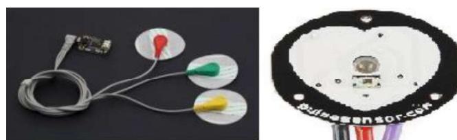
Figure 2.5: Gravity ECG Sensor (Left) and Arduino PPG Pulse Sensor (Right)
