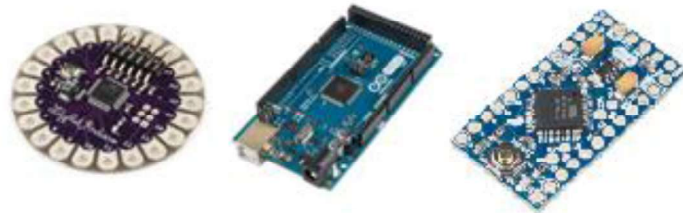
Figure 2.3: Arduino Microcontroller Boards (Left to Right: Lilypad, Arduino Mega, Arduino Pro Mini)
