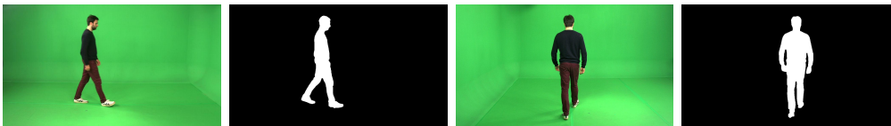
FIGURE 3.11: Background subtraction of a side view silhouette (left) and frontal view silhouette (right).
