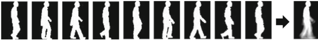
FIGURE 2.9: Gait sequence through a series of key silhouettes, and the resulting Gait Energy Image (GEI) [5]
