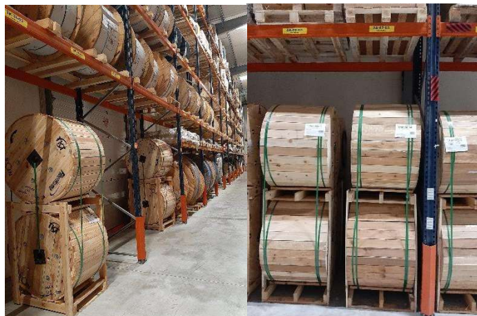
Figure 23 - Fibre-optic cable drums storage
