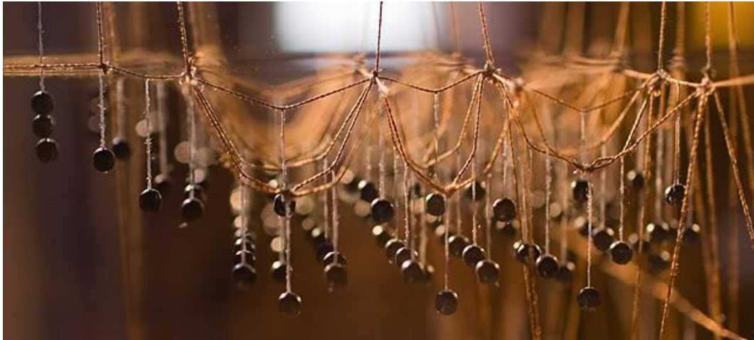
Figure 8.0:2. Gaudí's catenary arch 2 .
