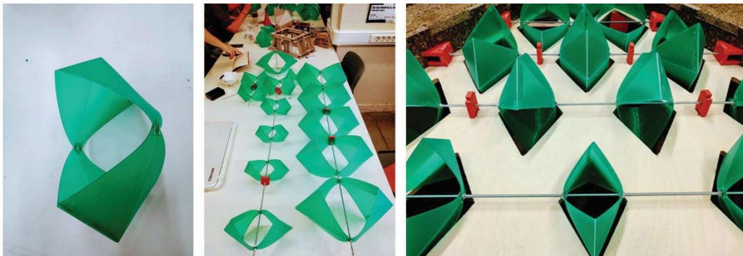
Figure 5.0:21. Bioshading unit's construction and assemblage.
