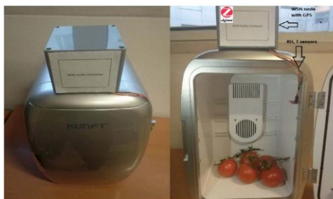
Fig. 8. Temperature and Humidity; measurement on simulated reefer container: tomato transportation case
