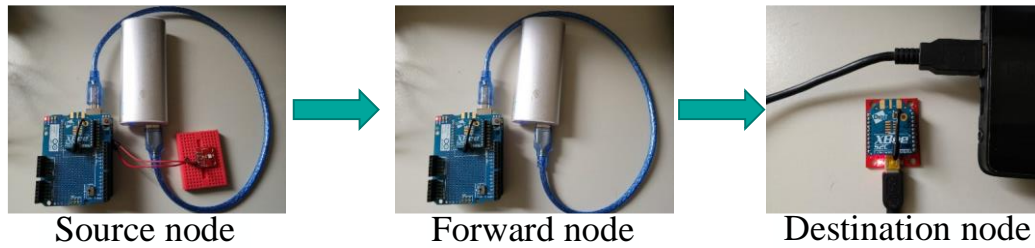
Figure 6.3 - Three XBee S2C node experiment diagram
