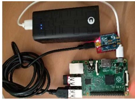
Fig. 6. The coordinator implementation: Raspberry PI 2 with WiFi, power bank, ZigBee Coordinator
