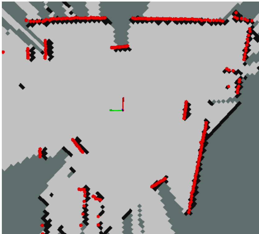
Figure 4.6 – LIDAR point cloud image using RVIZ tool
