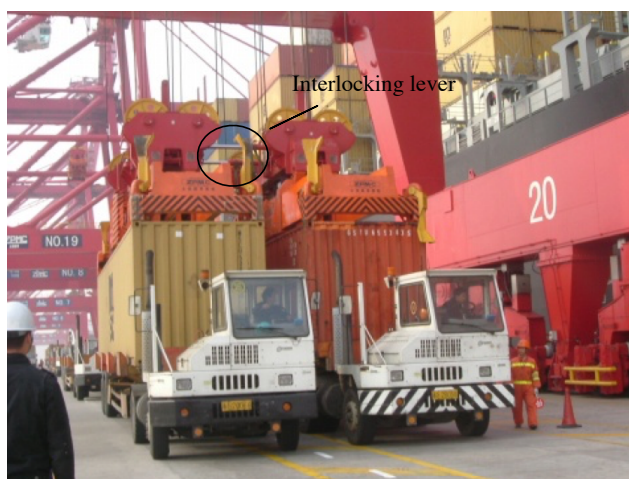
Figure 3.3 The double containers of overhead crane is working in interlock mode
