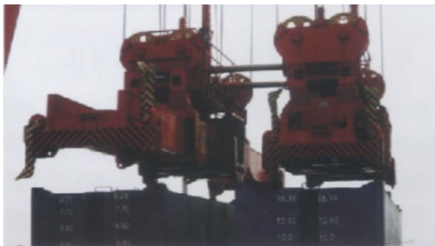
Figure 1.1 The double containers of overhead crane at the working place
