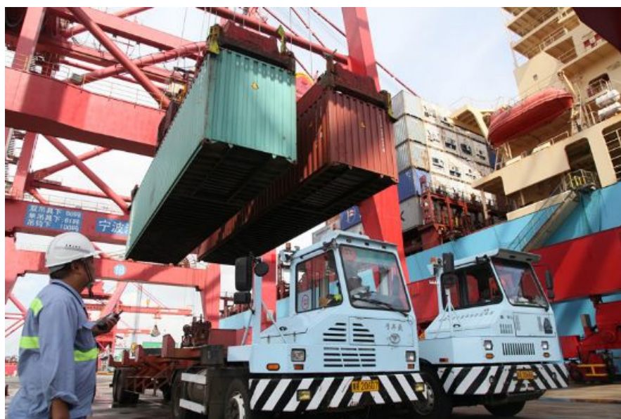
Figure 1.2 The double containers of overhead crane is working in unlock mode
